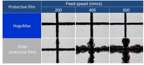
Process condition : 5.9W\_40kHz\_Just focus
