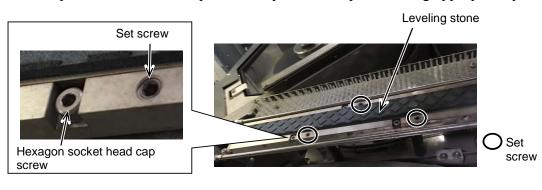
Step No. Procedure 1 Connect the handy panel at the Z1 side. 2 Move the brush of the washing unit to the washing (center) position. →Refer to Section 2-3-8, [Operation Screens for Washing Unit] of Chapter G in the Maintenance Manual for operation details of the washing unit. 3 Display the operation screen for the transfer arm 2. R #300 T.ARM2/ INITIAL T: ###.## ° VAC: ### kPa VACUUM ON **VACUUM OFF** INITIAL BLOW ON **BLOW OFF** SEQUENCE WATER ON WATER OFF
